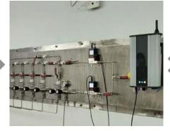
Lab Calibration Laboratory calibration is done in a controlled environment for all parameters to compensate for cross-sensitivity and ensure higher data accuracy.
