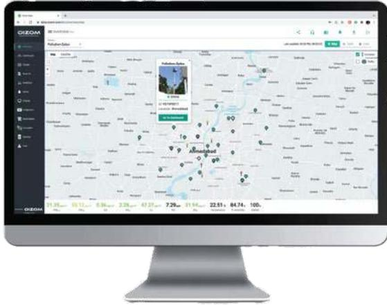
Envizom™ is an air quality monitoring software for real-time air quality data acquisition, visualization, and analytics. The Oizom® environmental data interpretation engine fetches the data from the Oizom® Environmental monitoring stations. On receiving the data, the engine runs necessary corrections and compensation algorithms. Envizom™ uses secured HTTPS servers for data storage. Alternatively, this data can also be stored on local servers.
