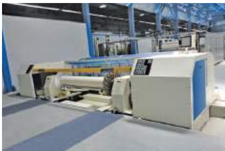
Textiles Industry Sizing process
