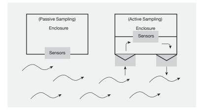
Sensor-based air quality monitoring systems have also evolved with technological advancements. Conventional sensor-based systems had their sensors exposed to ambient atmospheric conditions known as passive sampling-based sensors. Due to which, ambient environmental conditions such as heavy dust, high wind speed, temperature, and humidity affects directly exposed sensors. Such systems are highly affected by the above mentioned environmental con-
